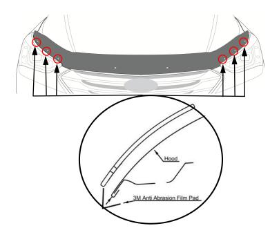
7. Peel and fold an anti-abrasion pad in half over the edge of the hood in alignment with the holes in the protector at the six locations over the headlights.
