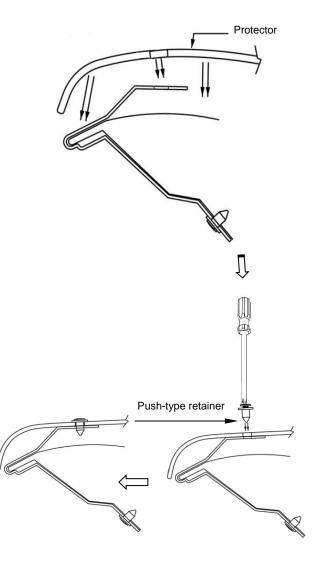
3. Install Metal Brackets over the anti abrasion film pads installed in the previous step. Align the hole in the bottom leg of the bracket with the round hole in the hood. See Illustration.
