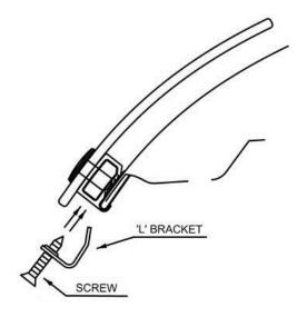
10. Insert a screw through an 'L'- bracket and into the clip body.
