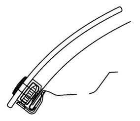
11. Make sure all the components are well seated together the protector is centered on the hood and then tighten the screws into the clips.
