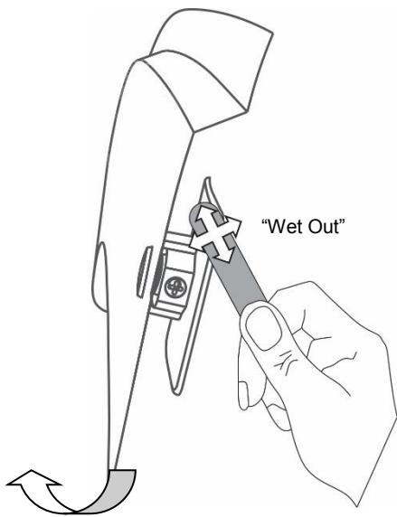
7. Gently lift visor away from door frame so the pull tab on the adhesive pedestal is accessible. Pull the protective backing from the pedestal and firmly press the visor onto the door frame. Using the wooden "wet-out" stick supplied, apply pressure to the surface of the adhesive pedestal. This will make sure there is maximum contact between the adhesive tape and door frame.
