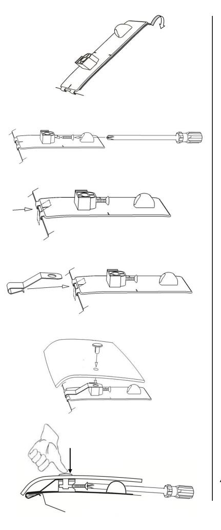
7. Remove the protective backing film from each of the adhesive pedestals and install them on the hood surface.
