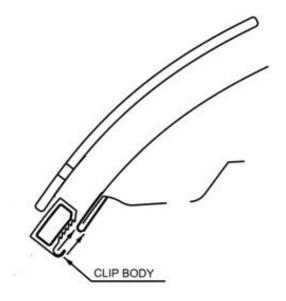
14. Place a clip body over each of the anti-abrasion film pads on the edge of the hood.
