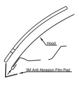
13. Peel and fold two (2) of the large anti-abrasion film pads in half over the hood edge aligned with the outer holes of the deflector in the area above the headlights.
