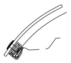
17. Make sure all the components are well seated together; the protector is centered on the hood, and then tighten the screws into the clip bodies.
