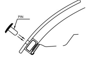
15. Insert a pin through the protector into each of the clip bodies.
