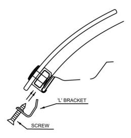
16. Insert a #6 x 5/8" screw through an 'L'- bracket and into the clip body.
