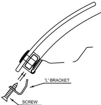
18. Insert a #6 x 5/8" screw through an 'L'- bracket and into the clip body.
