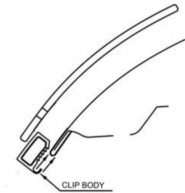
16. Place a clip body over each of the anti-abrasion film pads on the edge of the hood.
