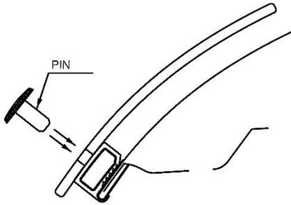
17. Insert a pin through the protector into each of the clip bodies.
