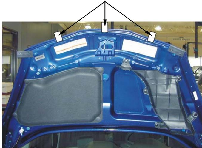
4. Install square plastic expansion plugs into the top of each of three (3) metal brackets, and two (2) adhesive backed pedestals.
