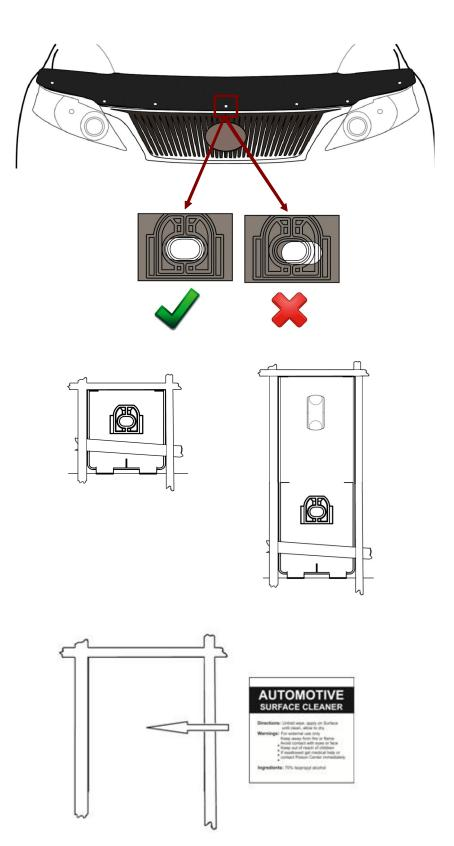
7. Confirm correct positioning of the pedestals, by adjusting the pedestal position on the hood to align with the holes in the hood protector.
