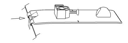
12. Peel and fold the small anti abrasion film pad in half over the hood edge between the fingers on the pedestal.
