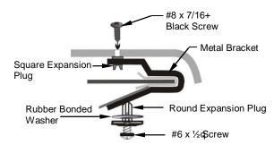
Install the remaining two (2) metal brackets (Type 1) over the hood edge, at 245mm location. See Illustration in step 3. Note: the #8 x 7/16" black screw and hood guard are not put in place until step 15.
