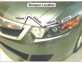
Open the hood. Peel and fold anti-abrasion film pads in half over the edge of the hood in the four (4) locations shown in the illustration below.
